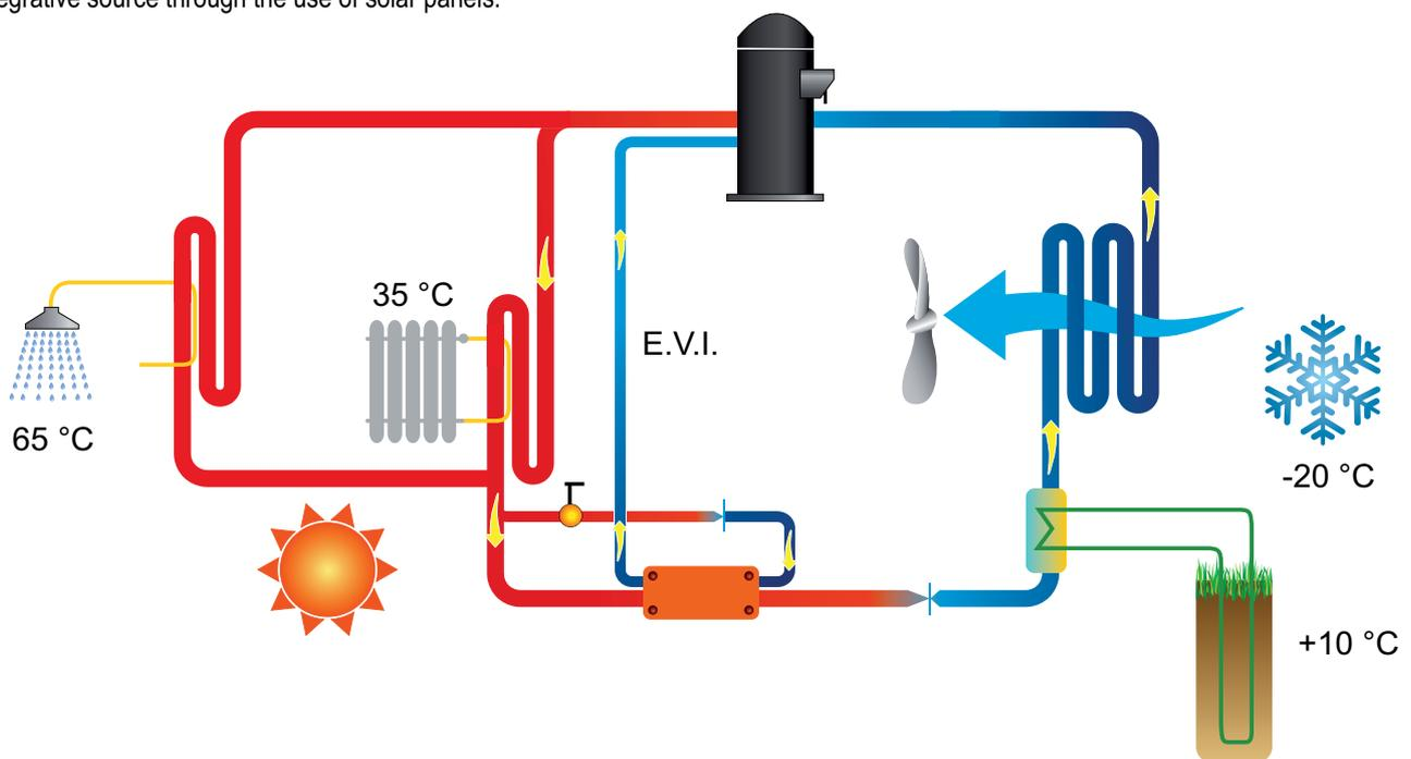
Refrigerant circuit layout of an LWZ/SW6 hybrid heat pump, supplied with domestic hot water heat exchanger and additional ground source heat exchanger to enhance the efficiency of the unit in case of severe ambient condition and to improve the seasonal C.O.P..
