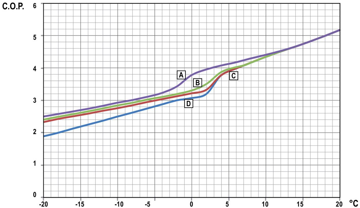
The graph shows the evolution of LWZ units C.O.P. (curves A, B, C) at different external temperatures (with user water produced at 35 °C), compared to a unit of equal power series LZT (curve D).
